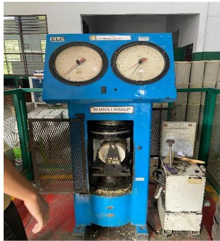
Gambar L.1.16 Mesin Compression
