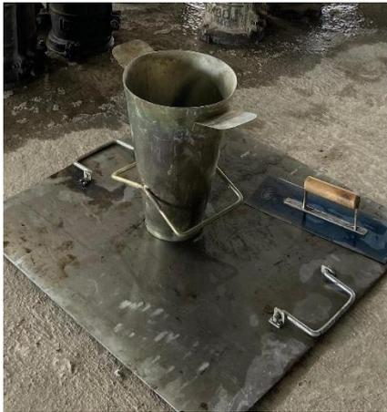
Gambar L.1.3 Kerucut Abrams
