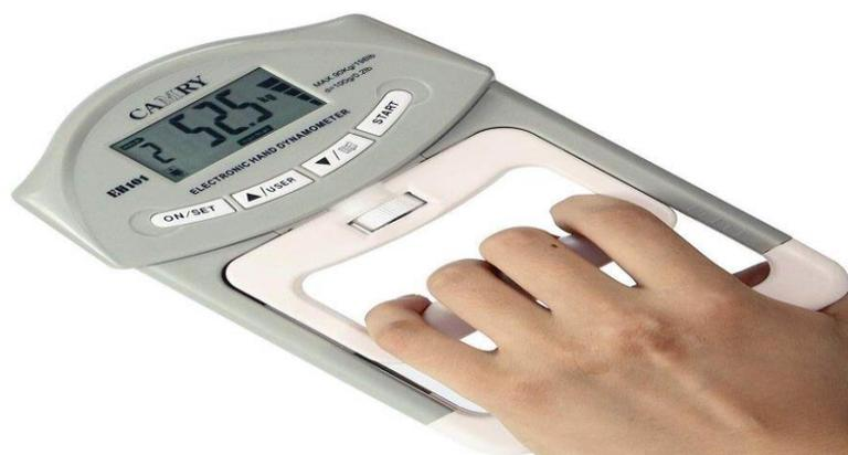
**Gambar 2.6** Hand Grip Dynamometer
