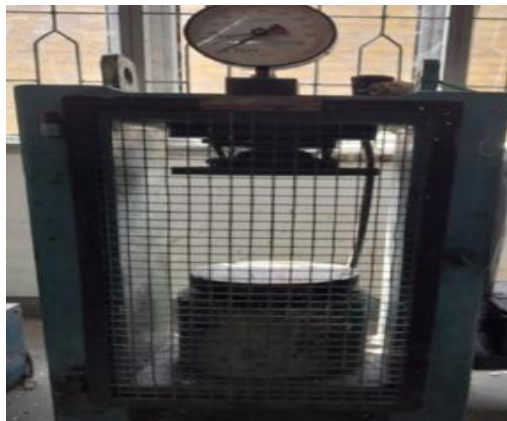
Gambar 3.19 : Alat Penguji Beton compression machine test
