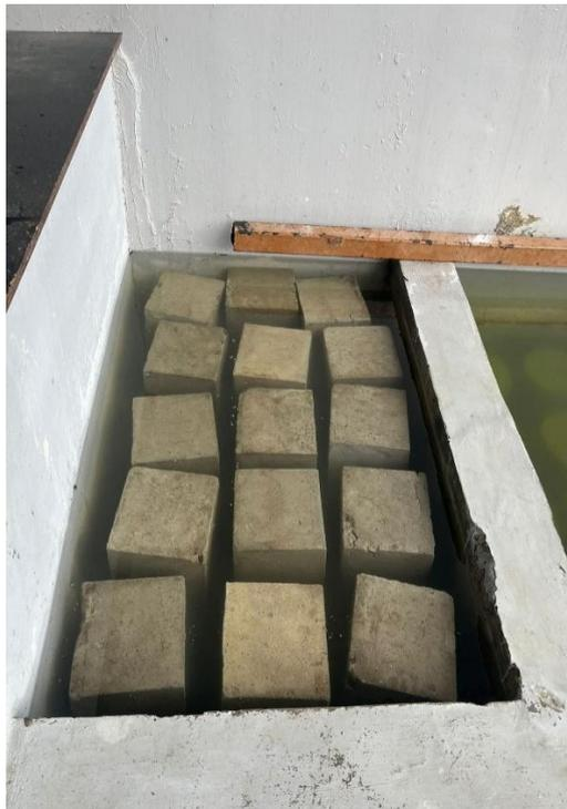
Gambar L.4: Perendaman benda uji balok.
