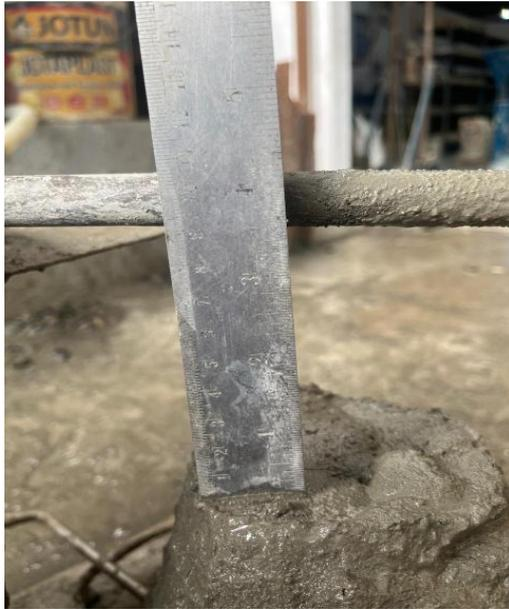
Gambar L.3: *Slump test*
