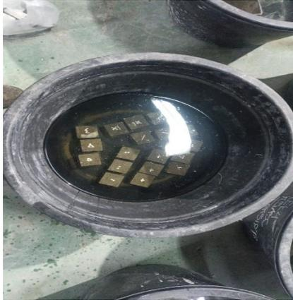
Gambar L. 16 Perendaman Benda Uji Mortar
