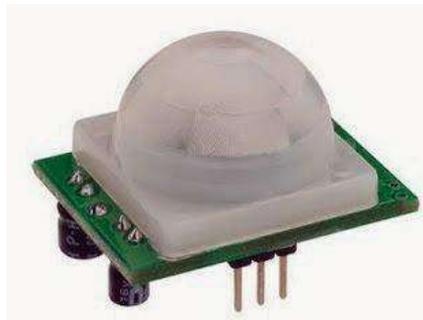
**Gambar 2.2. Sensor PIR (*Passive Infrared Receiver*)
