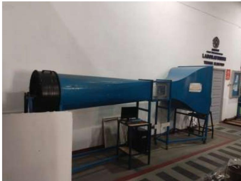
Gambar 2.9 *Wind tunnel*
