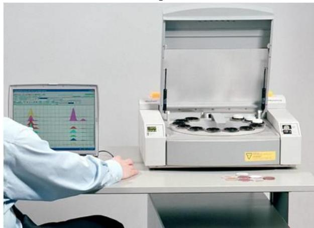
Gambar 3.4 *X-Ray Fluorescence (X-RF)*
