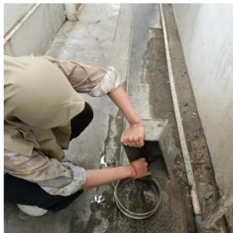
Gambar L. 4: Pengujian kadar lumpur agregat halus.
