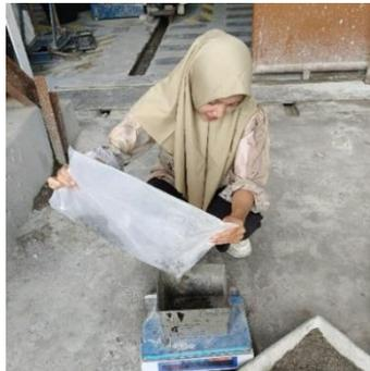
Gambar L. 3: Pengujian kadar air agregat halus.
