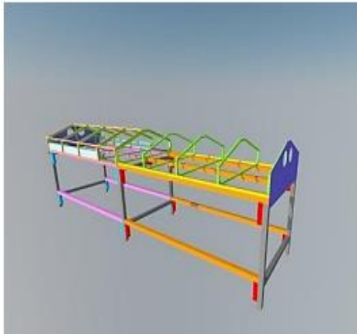
Gambar 2. 5 Solar Tunnel Dryer (Khatir R et al., 2021)
