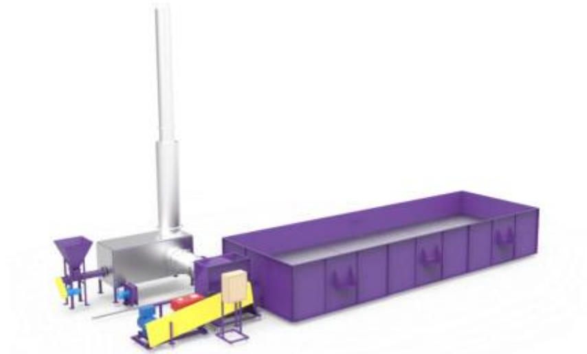
Gambar 2. 3 Flatbed Dryer (Dandy Z et al., 2022)
