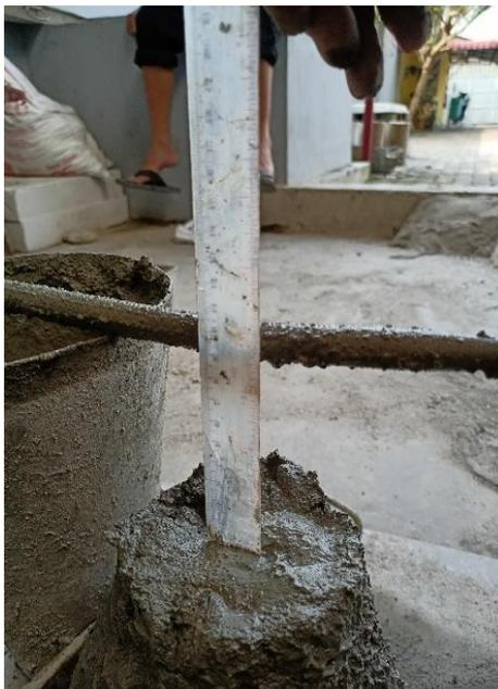
Gambar L – 6: Pengecekan Slump.
