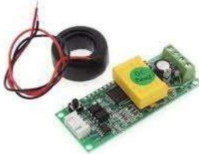
**Gambar 2.2** Sensor PZEM-004T (Sumber : <https://encrypted-tbn0.gstatic.com/>)
