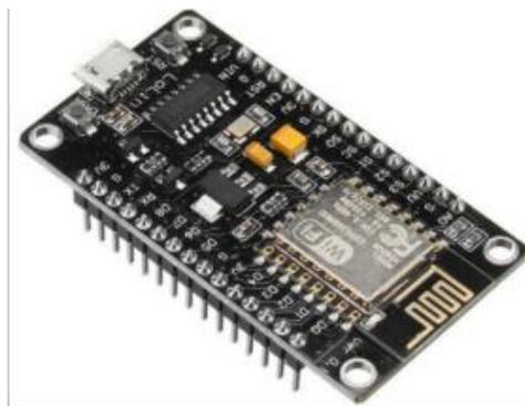
**Gambar 2. 3** NodeMCU V3
