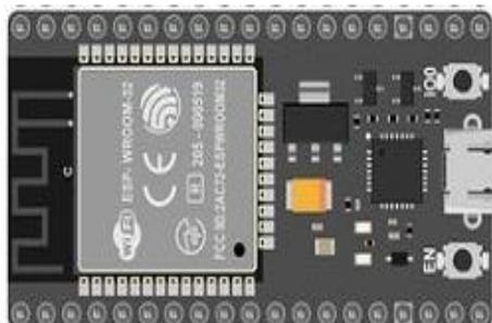
Gambar 3.1 NodeMCU ESP32
