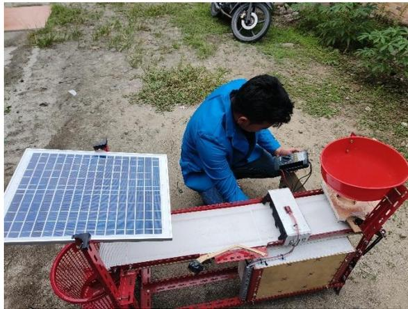
Gambar 1. Menganalisa Tegangan Input / Output Solar Panel
