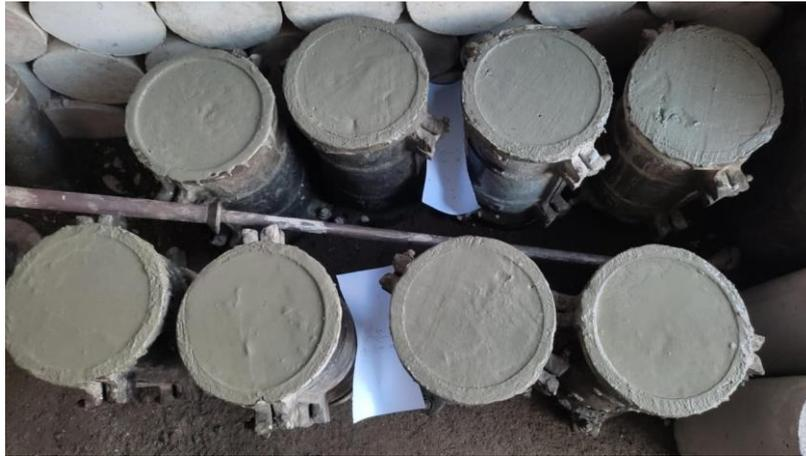
Gambar L. 12 Sampel Beton Segar
