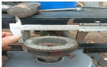
Gambar 4.1 Mengukur pulley motor
