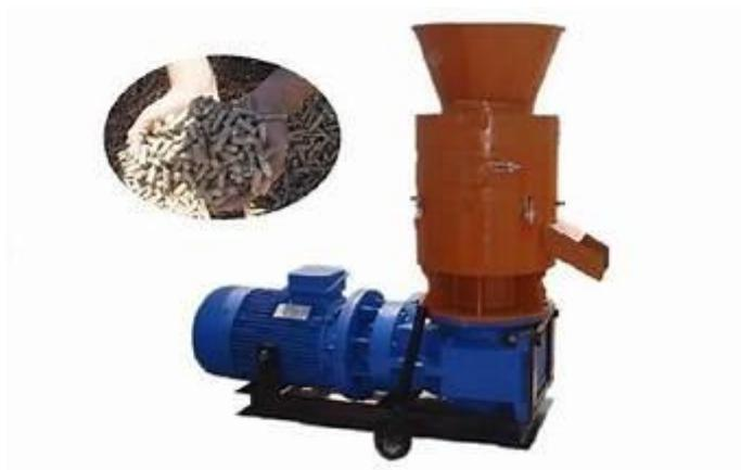
Gambar 2.1 Mesin Biomass Pelet Kayu
