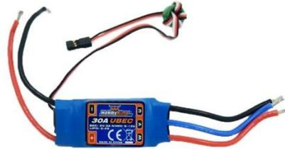
Gambar 2. 7 Electronic Speed Controller
