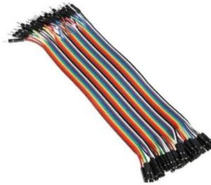
Gambar 2. 11 Kabel Jumper
