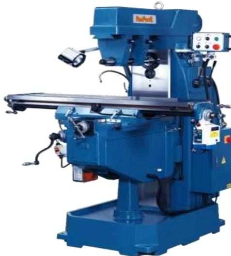
Gambar 2. 13 Mesin *Frais Horizontal*
