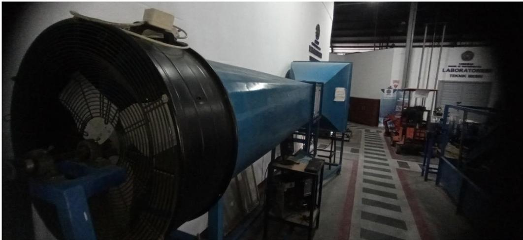
Gambar 2. 1 *Wind Tunnel*
