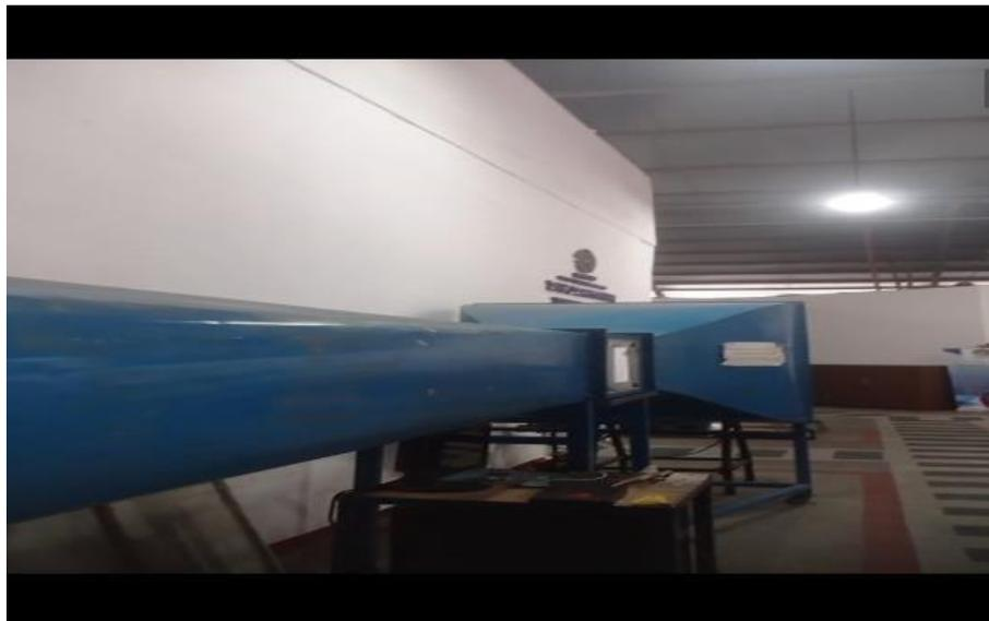
Gambar 3. 3 Wind Tunnel
