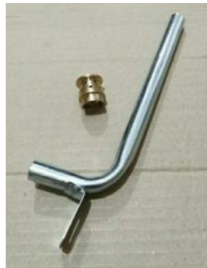
Gambar 2.6 Pipa Burner (Adi et al. 2014)
