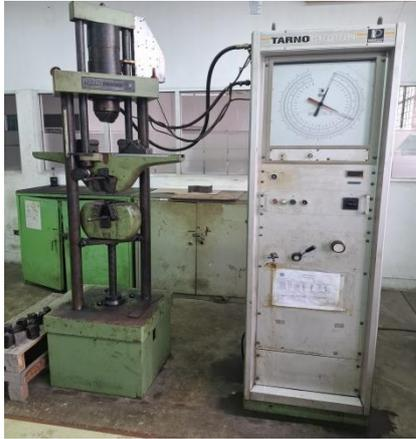
Gambar 3.15 Mesin Uji Tarik (*Universal Testing Machine (UTM)*)
