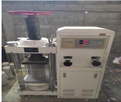
Gambar alat 21: CTM (Compression Testing Machine)
