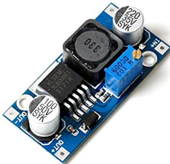
Gambar 2.10 Modul penaik tegangan DC to DC XL 6009.
