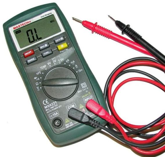
Gambar 2. 19 Multimeter digital
