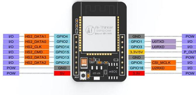
**Gambar 2. 2 Pinout ESP-32CAM**
