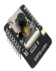
Gambar 2. 2. ESP32-Cam
