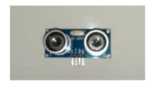
Gambar 2. 9. Sensor Ultrasonik HC-SR04
