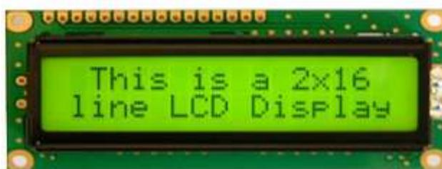
Gambar 2. 13 LCD 2x16
