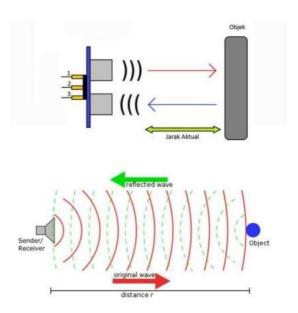
Gambar 2.5. Cara Kerja Sensor Ultrasonik Dengan Transmitter Dan Receiver Yang Terpisah (Sukmana, 2019)
