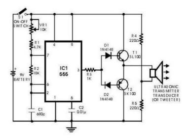
Gambar 2.6. Rangkaian Dasar Dari Transmitter Ultrasonik (Karmia, 2019)
