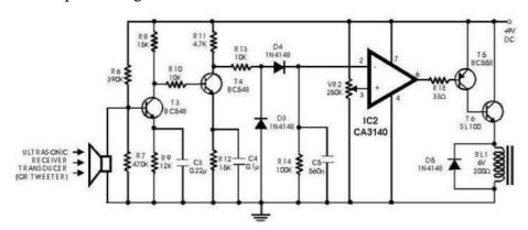
Gambar 2.7. Rangkain Dasar Receiver Sensor Ultrasonik (Karmia, 2019)
