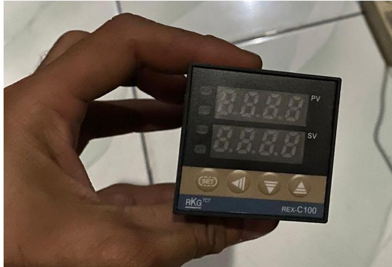
Gambar 4.25 Thermostat Suhu Controller
