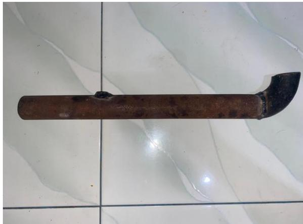
Gambar 4.15 Pipa Burner
