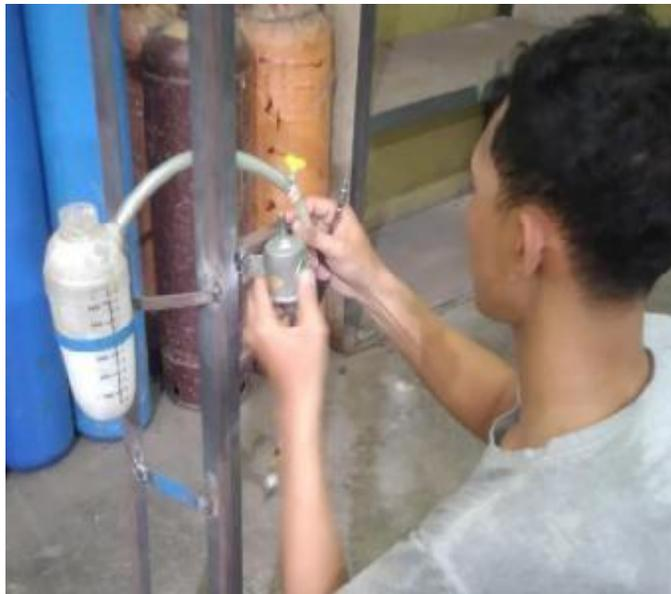
Gambar 4.21 Pemasangan electric fuel pump
