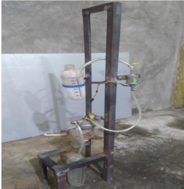
Gambar 4.25 Hasil perakitan oil water separator
