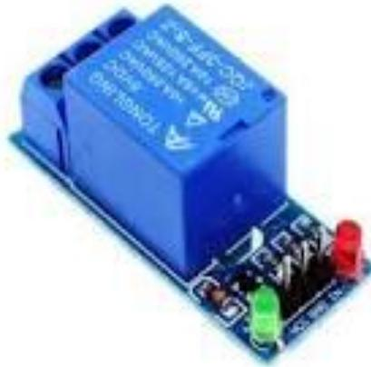
Gambar 2.14 Relay 1 Channel
