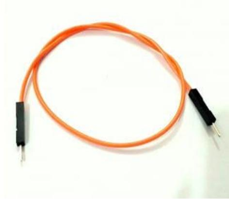
Gambar 2.24 Kabel *Jumper Male to Male*
