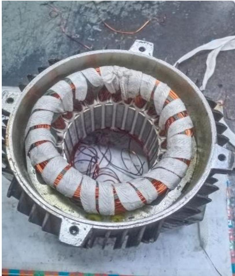
Gambar 4.15 Pengikatan winding stator.
