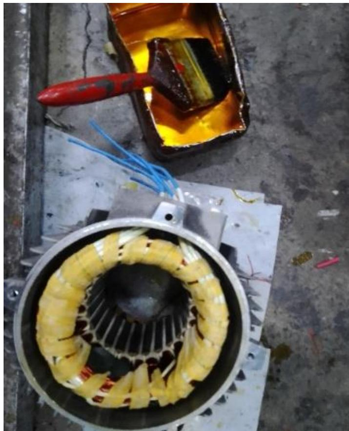
Gambar 4.16 Proses varnishing
