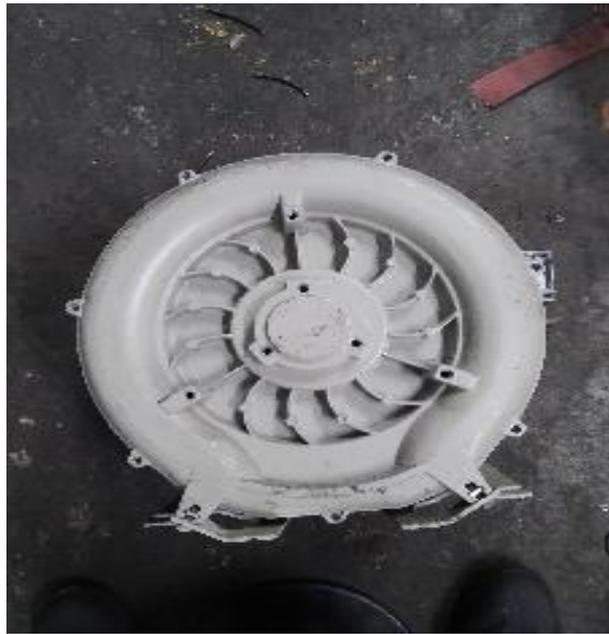
Gambar 4.2 Cover Impeler Motor
