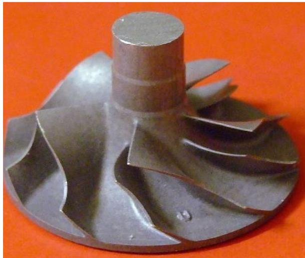
Gambar 2. 5 Titanium alumida
