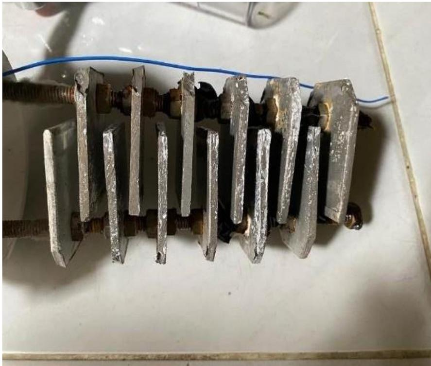
Gambar 3. 1 Elektroda Plat Titanium
