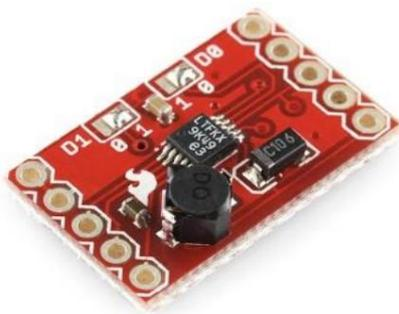
Gambar 2.34 Energy Harvester Module
