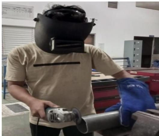
Gambar 4.2 Memotong Pipa
