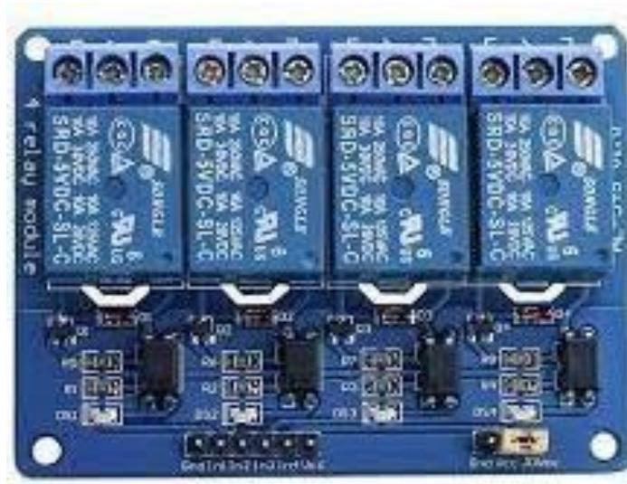
Gambar 2.5 Modul Relay 4 Channel
