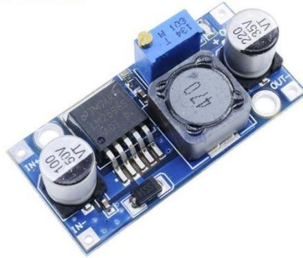
Gambar 2.6 LM2596 DC-DC StepDown LM2596 DC-DC
