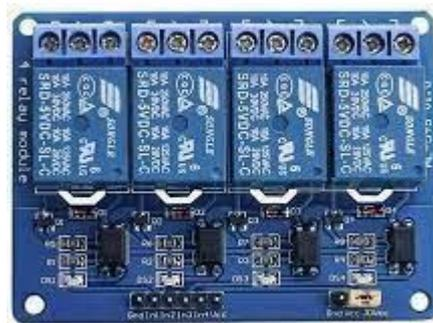
Gambar 3.7 Modul Relay 4 channel
