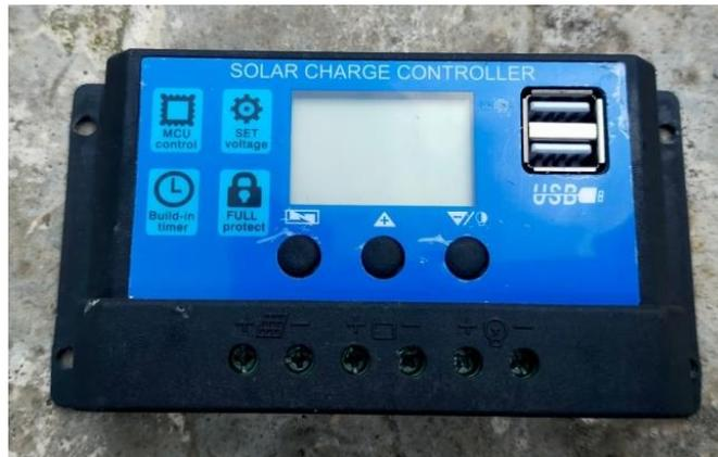
Gambar 2. 4 Solar Charge Controller
