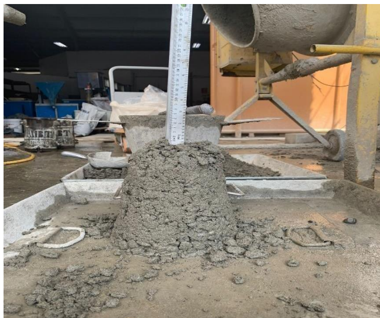
Lampiran 6: Pengujian Slump
