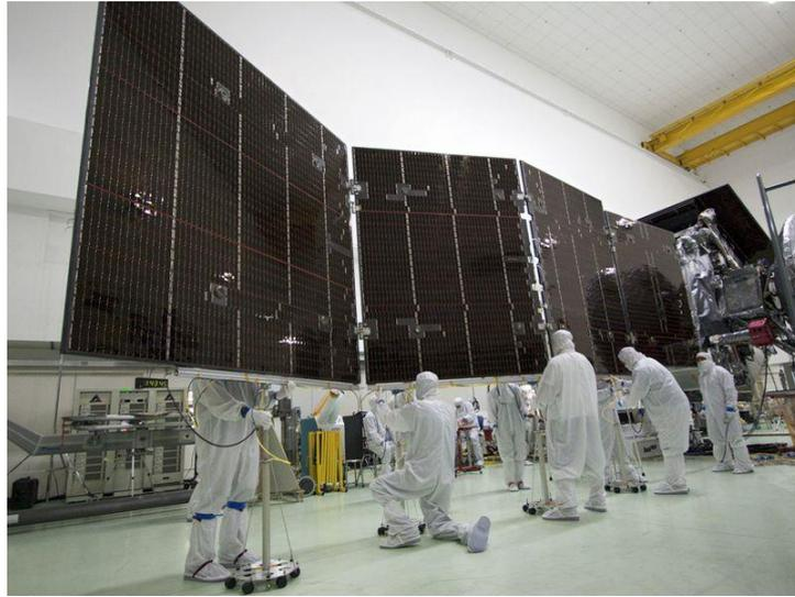
Gambar 2.4. *Compound Thin Film Triple Junction Photovoltaic*
