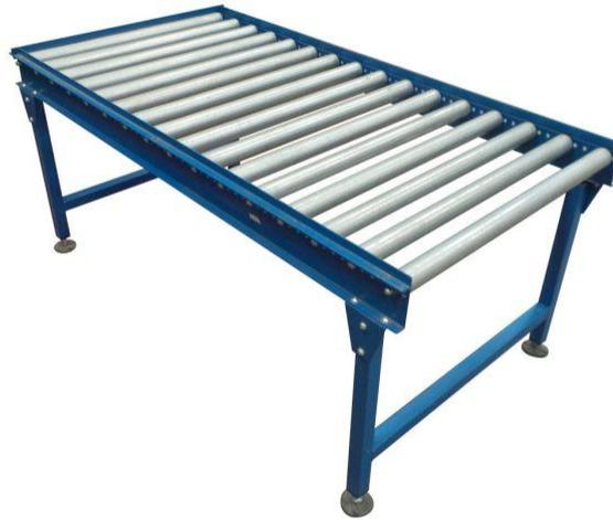
Gambar 2.12. Frame Conveyor Otomatis
