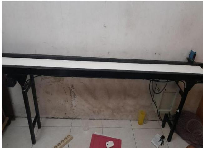
Gambar 4.15. Conveyor Otomatis Sudah Terpasang Panel Dan Sensor
