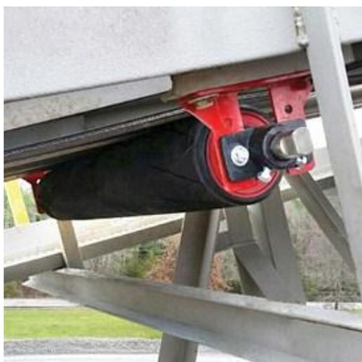
Gambar 2.3. Idler Conveyor Otomatis
