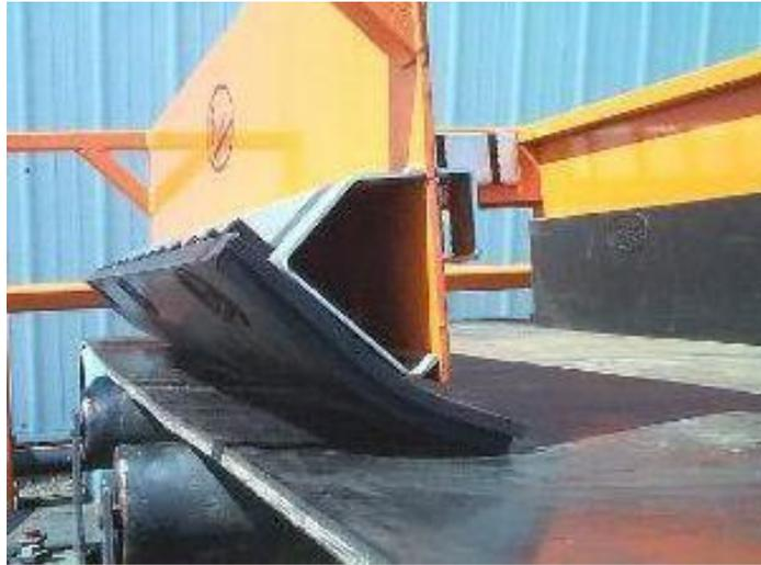
Gambar 2.10.Skirt Conveyor Otomatis
