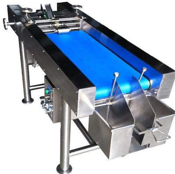
Gambar 2.7. Feeder Conveyor Otomatis
