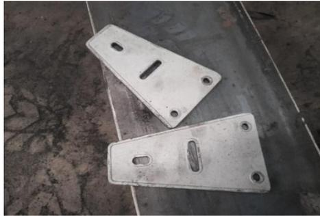
Gambar 4. 3. Sapot Frame Dan kaki Conveyor Otomatis
