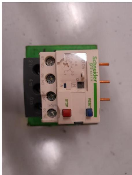
Gambar 2.16. Thermal Overload Relay
