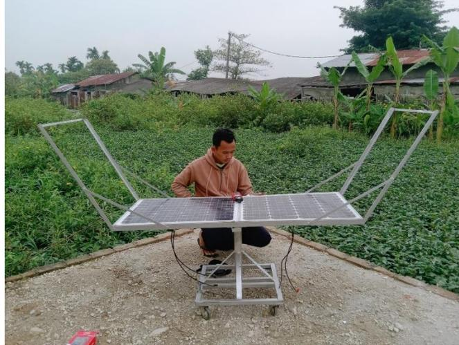
Gambar 1: Pengukuran Panel surya Tanpa Kaca film
