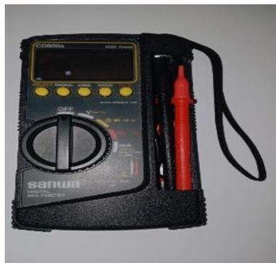
Gambar 3.1: Alat ukur multimeter digital
