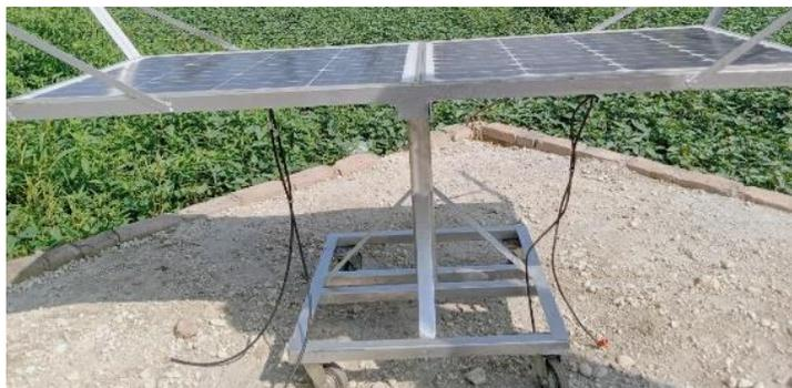
Gambar 3.6: Kerangka Panel Surya
