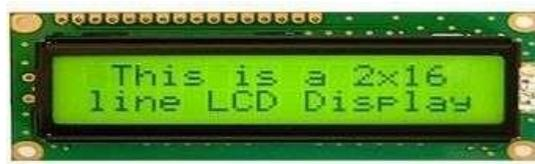
Gambar 2.12 Liquid Crystal Display
