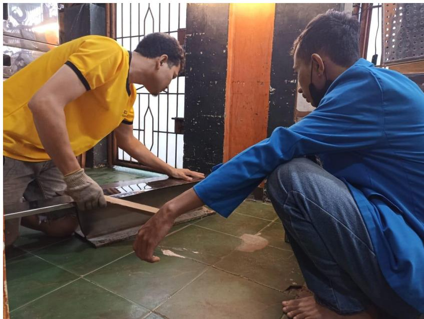
Gambar 4.3. Proses Pelekatan Dinding Stainless Steel
