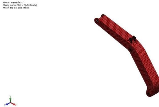
Gambar 4.3 Hasil Proses *Meshing Boom*
