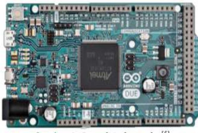
Gambar 2.3 Arduino Due
