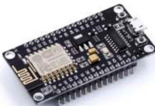
Gambar 2.8 NodeMCU ESP8266
