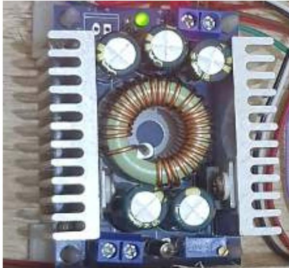
Gambar 3.7 Buck Boost Converter DC-DC
