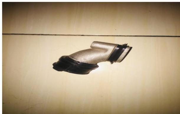
Gambar 2.7 *Intake Manifold*
