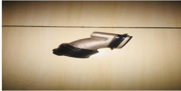
Gambar 3.18 *Intake Manifold* Standar
