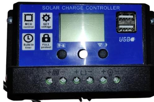
**Gambar 2.15. Solar Charge Controller**
