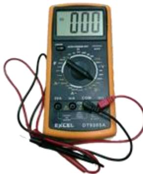
**Gambar 3.4. Multimeter Digital**
