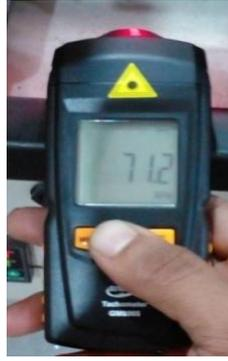
Gambar 3. 9 Tachometer GM8905
