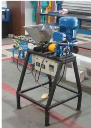
Gambar 3. 1 *Conventional single screw extruder*
