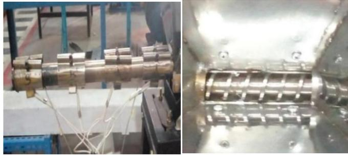
Gambar 3. 2Barrel & Screw
