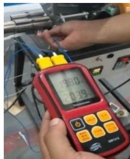
Gambar 3. 8 Thermometer Digital GM1312
