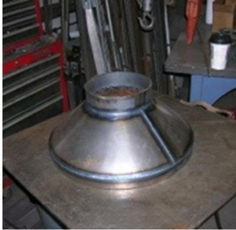
Gambar 2.10 Cerobong Asap ( Chimney ) (Sumber: Fathurohman, 2015)
