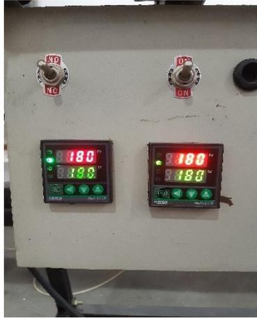
Gambar 3.17 *proportional integral derivative* (PID)
