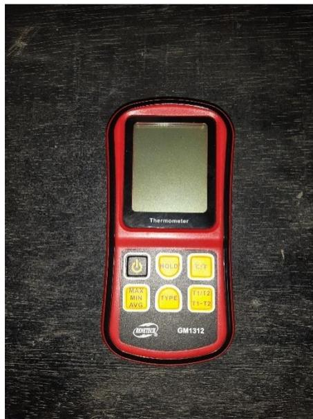
Gambar 3.9 Digital Thermometer Benetech GM 1312
