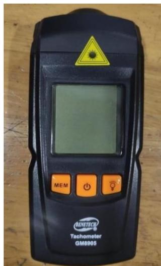
Gambar 3.8 Digital Tachometer Benetech GM 8905
