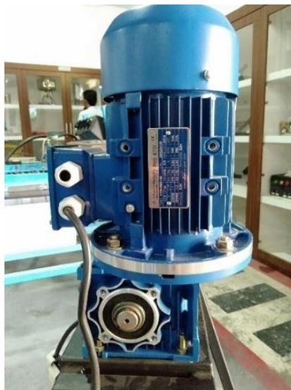
Gambar 3.4. Motor Gearbox
