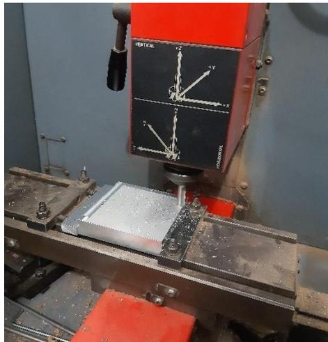
Gambar 4.2 Proses Milling Pada Mesin T.U CNC-3A
